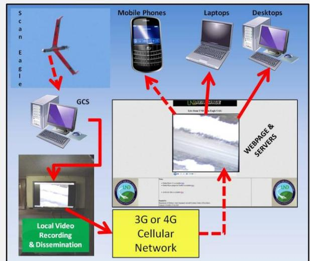
Flow diagram of video streaming from the ScanEagle UAS during deployments (dashed lines are wireless links).
