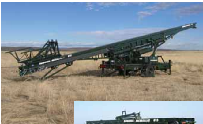
MC255LLR Launcher (ready to launch & transport configuration) Robonic, Finland
