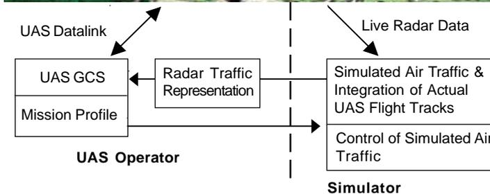
Emergency procedures for disrupted data link between UAV and GCS: Since UAS are controlled by distant operators via data link, it must be assured that a disruption of the data link connection does not result in an uncontrolled UAS and thus compromise safety. Internationally binding procedures that prescribe the safe termination of a UAV mission, for example, UA self-destruction or automatic landing at the next airfield must be developed.
