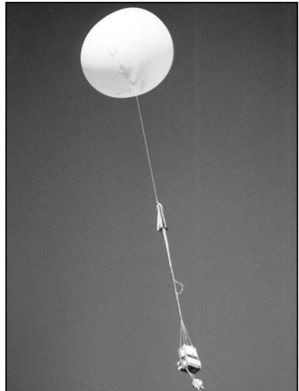
This High Altitude Balloon Group launch on August 19, 2002 carried instruments to detect mercury in the upper atmosphere. The payload was contained in a homemade styrofoam beer cooler. The balloon is shown here shortly after launch when it was six feet in diameter. At maximum altitude the balloon was 60 feet in diameter.
